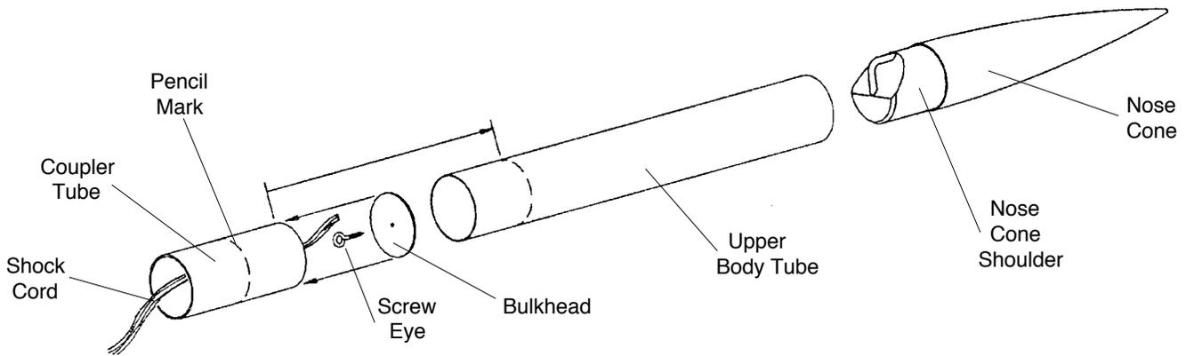
1. Paint the back 12-7/16" (31.6 cm) of the upper body tube white. Paint the rest of the tube and the nose cone a shade of red that matches the red of the decal sheet.
