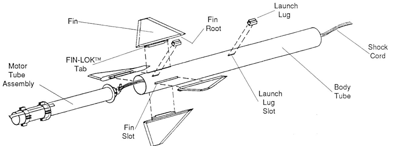
1. Using a hobby knife, carefully remove any body tube material that may still be attached to any pre-cut slots in the body tube.
