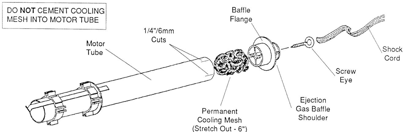
1. Make four 1/4" (6mm) long cuts, 90 degrees apart, in the front end of the motor tube.
