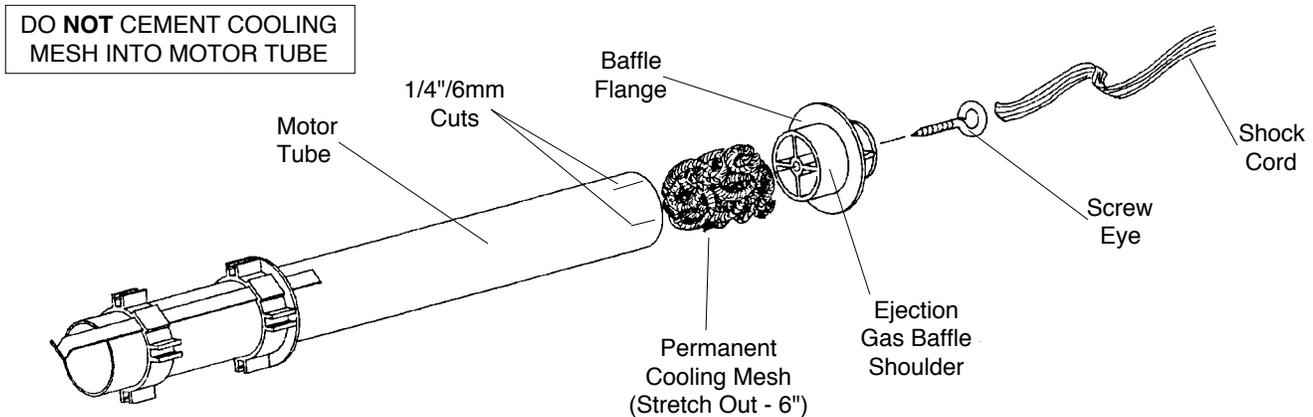
1. Make four 1/4" (6mm) long cuts, 90 degrees apart, in the front end of the motor tube.
