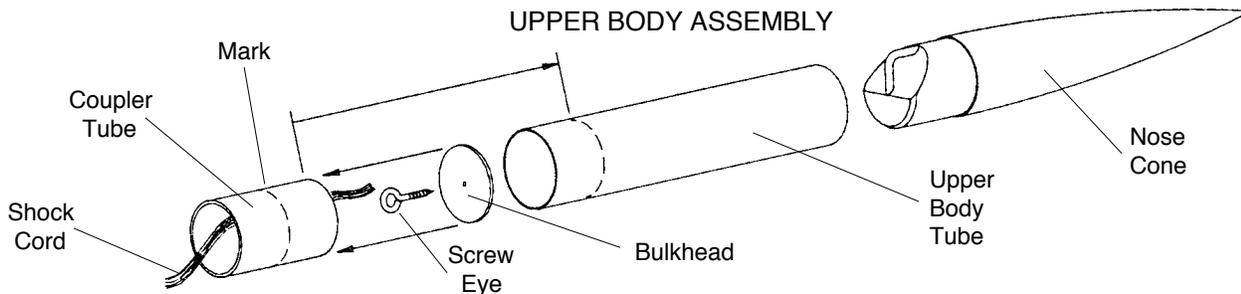
1. Screw the other screw eye all the way in to the hole in the bulkhead (1/16"/1.6 mm thick). Apply a bead of cement where the screw eye meets the bulkhead.
