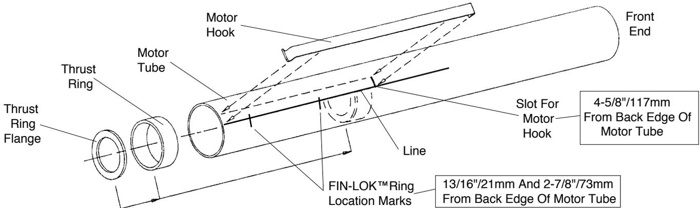
1. Cement the thrust ring flange (1/16"/1.6 mm thick) to the thrust ring (7/16"/11 mm long). Set the thrust ring assembly aside to dry.
