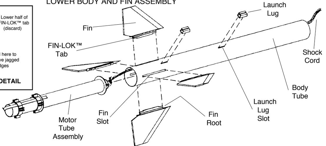
1. Using a hobby knife, carefully remove any body tube material that may still be attached to any pre-cut slots in the body tube.
