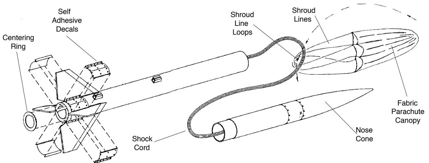
1. Slide the other centering ring over the back of the motor tube and motor hook and push it against the back FIN-LOK™ ring. Apply a bead of cement where the centering ring meets the body tube.
