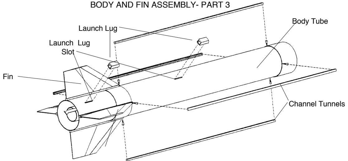
1. Wrap the channel tunnel marking guide around the body tube making sure to line up the alignment arrows with the fins. Using a pencil or pen, make marks at the arrow points shown on the strake marking guide. Remove the marking guide and using a straight edge, connect the marks made on the tube along the length axis.
