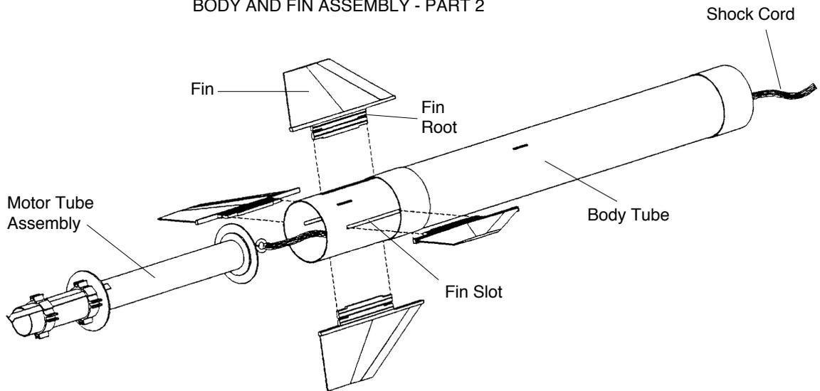
1. Insert the loose end of the shock cord and then the motor tube assembly into the back of the rocket body tube as shown. Position the motor tube assembly so that the fin locks are located under and visible through the body tube's pre-cut fin slots.
