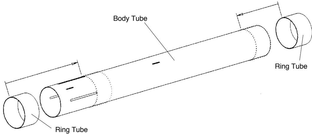
1. Using a hobby knife, carefully remove any body tube material that may still be attached to any pre-cut slots in the body tube.
