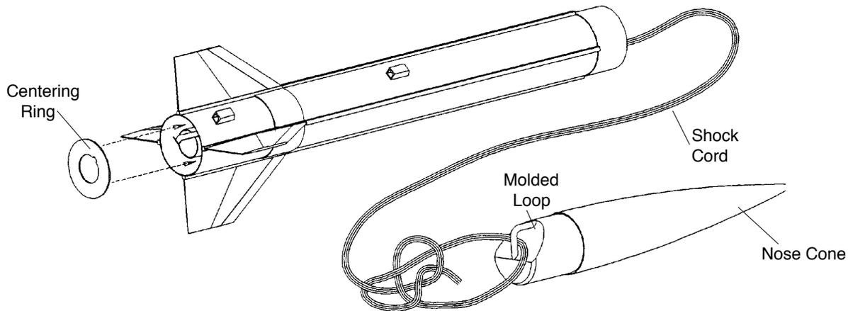
1. Slide the remaining centering ring over the back of the motor tube and motor hook and push it against the back FIN-LOK™ ring. Apply a bead of cement where the centering ring meets the body tube.
