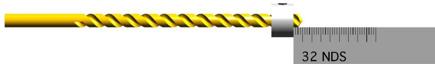
Using a stop collar or multiple wraps of masking tape, set the depth required using a machinist scale, 1/32" exposed drill bit tip per second shorter delay time desired than existing delay time.
